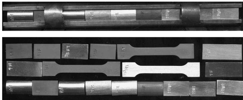
Fig. 2. Specimens of selected materials before insertion into one of the four specimen holders.
